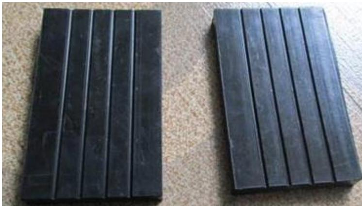
[Railway rubber pad](#) is an important part of track structure. It is installed between rail and concrete soft pillow. Its main function is to buffer the vibration and impact produced by vehicle passing through the rail, protect the roadbed and soft pillow, and insulate the signal system. As the rubber pad is exposed to the atmosphere for a long time, it is required to have good resistance to natural aging, cold resistance, heat resistance and corrosion resistance.
